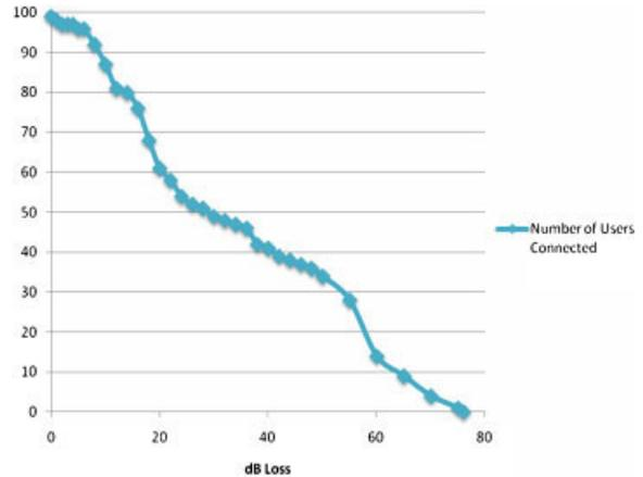
Fig. 4. Number of connected users *versus* loss in dB for the case of mountains signal loss.
