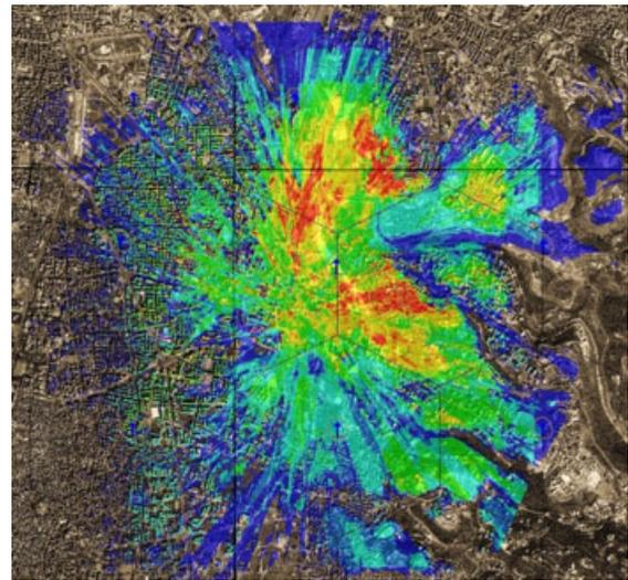
Fig. 9. Placing base stations in appropriate locations to get the highest percentage coverage.
