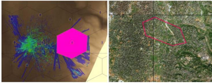
Fig. 8. Selection of a perfectly hexagonal area in pink (left) due to high building density. Selection of an extended area in pink (right) due to free space, thus an extended coverage capability by the BS.
