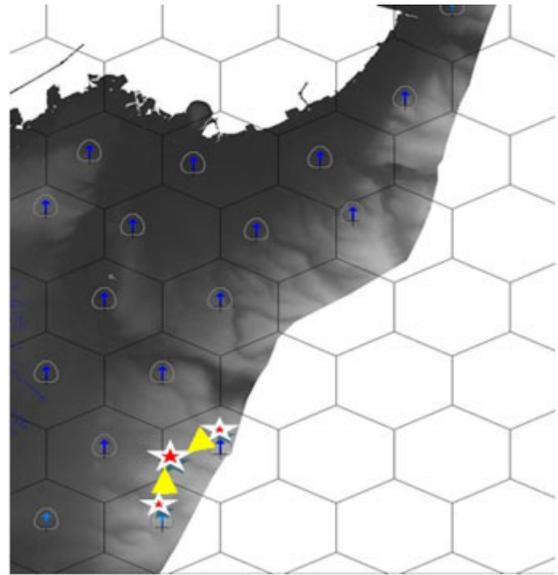
Fig. 6. Example of substituting every pair of base stations on the edge by a single BS.
