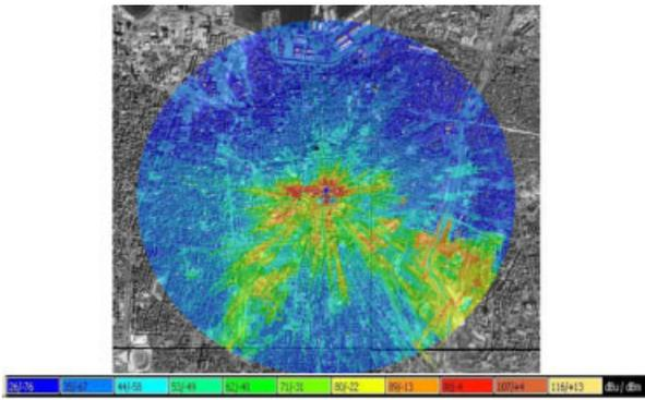
Fig. 1. Case where indoor loss parameters are not taken into account, 0 dB loss
