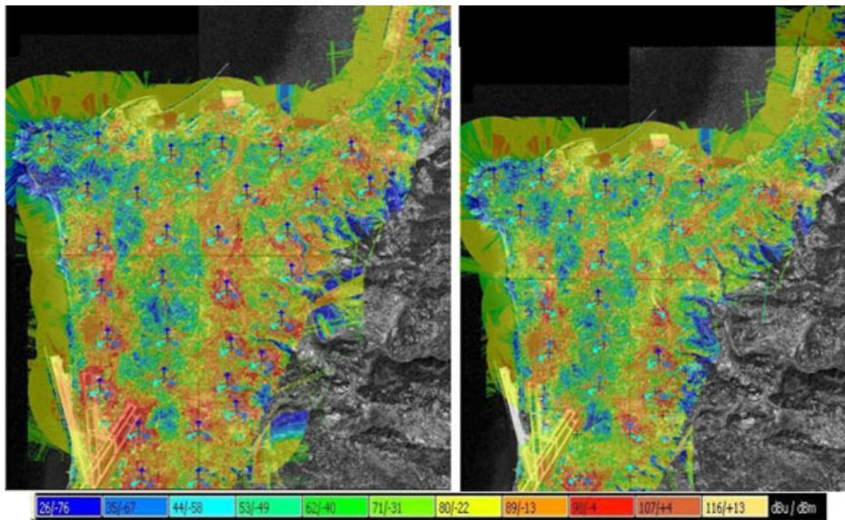
Fig. 10. Left side shows the coverage with 37 base stations, while the right side shows the coverage with 33 base stations.
