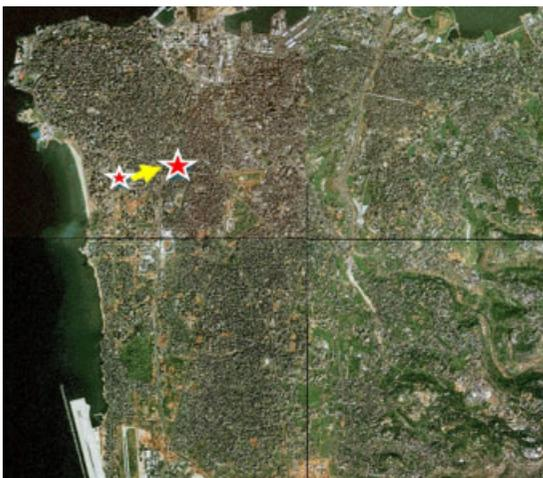
Fig. 5. Moving a base station from a location at the sea edge inland orthogonally to the sea edge. The small star shows the old BS location, whereas the big star shows the BS's new location.
