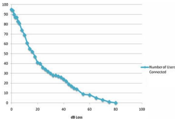
Fig. 3. Number of users connected *versus* dB Loss for the case of In-Building Loss.
