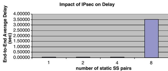
Fig. 20. IPsec impact on delay when many to 1 SS are connected for the 1TuM mode.
