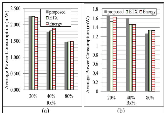
Figure 4. Average Power Consumption for 25 nodes (a) random deployment, (b) grid deployment
