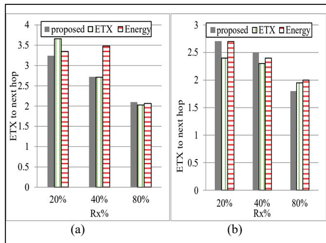
Figure 6. ETX to next hop for 25 nodes: (a) random deployment, (b) grid deployment
