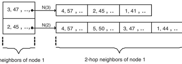
Fig. 3. Node 1 data structure.  $N(3)$  and  $N(2)$  represent the neighbors of nodes 3 and 2 respectively. The nodes are sorted according to their weights. Such a data structure enables node 1 to know its 1-hop and 2-hop neighbors.
